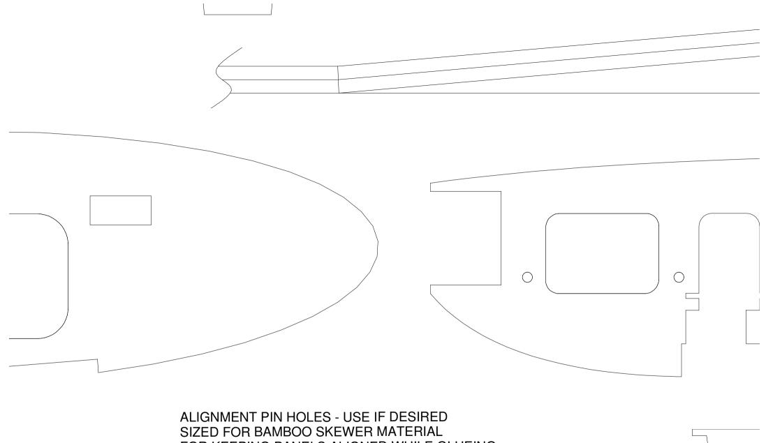
FOR KEEPING PANELS ALIGNED WHILE GLUEING
